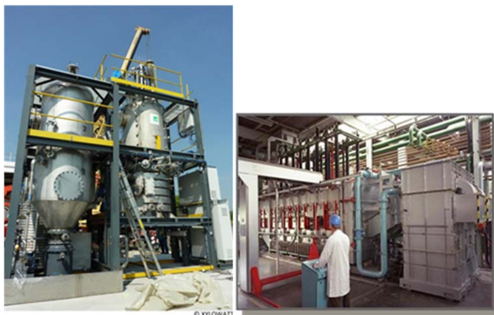
Figure 5 - Biomass gasifier and combustion test cell for BioVive Project
